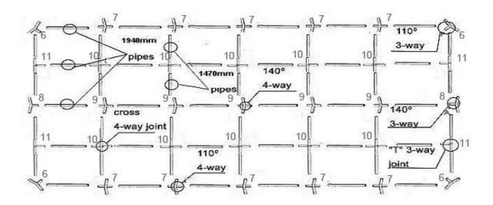
2. Connect pipes together starting with the center frame. Then assemble each side.
