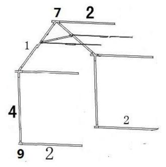
2. cover the roof on the top frame, and sidewall and endwall like 3X4M basic section. Add more expansion section to make your tent more bigger.
