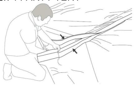
3. Attach one end of the support poles (4) to the roof joints (6,7).
