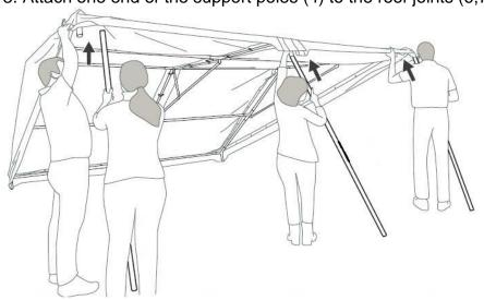
**4.** Attach the other 4 supporting poles (4) to the joints (5,6), build-up the framework .Use the 6x180mm peg to fix each pole into the ground and use the hook to fix the leg cover to the leg.
