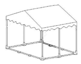
5. Spread the wall and door panels, and attach to framework using the bungee cords. Clasp the frame to the metal eyelets (located over the wall and door panels) to ensure stability. Also use the 4x180mm pegs to fix the doors and walls to the ground.
