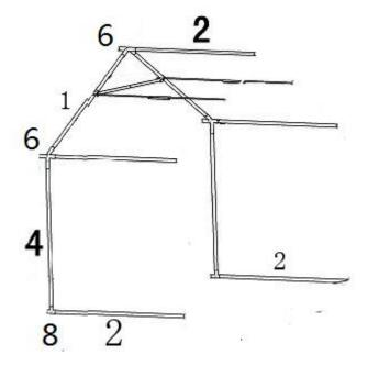
2. cover the roof on the top frame, and sidewall and endwall like 4X4M basic section. Add more expansion section to make your tent more bigger.
