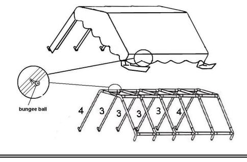
V spread the wall panel and door panel attach to framework by using the bungee cords clasping the frame to grommets that is construct over the wall panel and door panel to ensure stability. Also use the short pegs to fix the doors to the ground.
