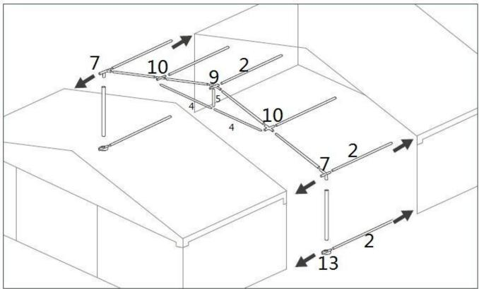
2. cover the roof on the top frame, and sidewall and endwall like 5X4M basic section. Add more expansion section to make your tent more bigger.
