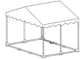
5. Spread the wall and door panels, and attach to framework using the bungee cords. Clasp the frame to the metal eyelets (located over the wall and door panels) to ensure stability. Also use the 4x180mm pegs to fix the doors and walls to the ground.
