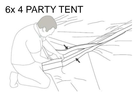
3. Attach one end of the support poles (3) to the roof joints (6,7).
