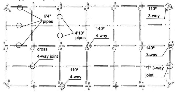
2. Connect pipes together starting with the center frame. Then assemble each side.
