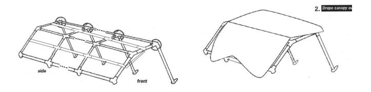
Insert the remaining legs and finish attaching cover to frame.
