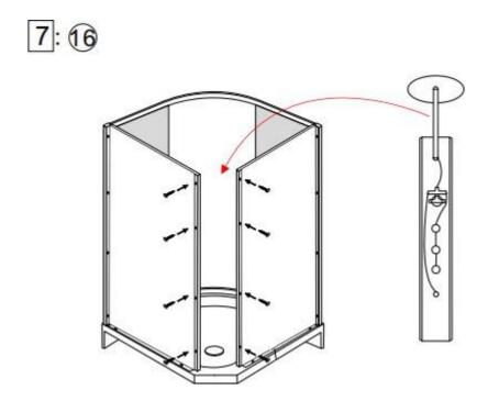
Connect the rear side panels to the middle section by drilling the screws in. Keep in mind that there are no pre-existing screw holes on the middle section.
