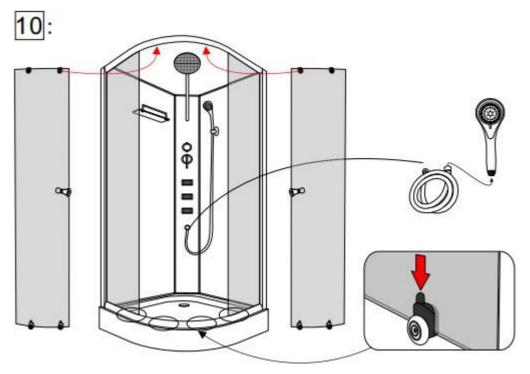
Attach the front glasses to the frame. Hang the top wheels on the top curved rail. Insert the bottom wheels into the bottom curved rail by pushing button.
