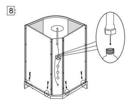
Secure the rear side panels to the base by screwing them in place. It uses the same method as attaching the panels to the base.
