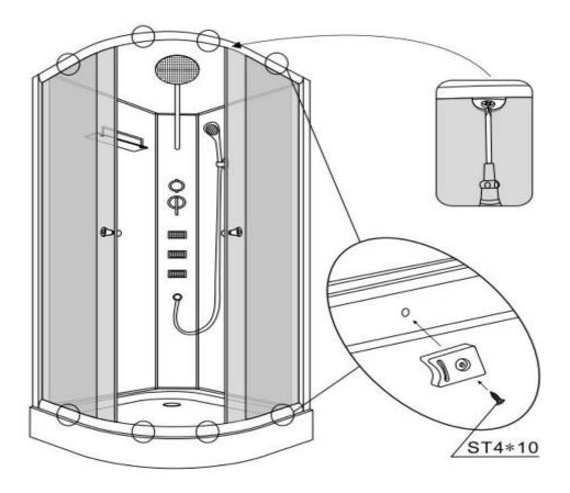
Attach the panel fixers to lock the glass panels.
