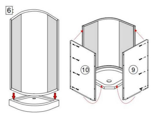
Put the front frame and two rear side panels on top of the shower tray. Attach the rear side panels to the front frame.
