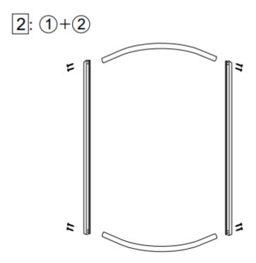
Join the curved rails with the side poles.
