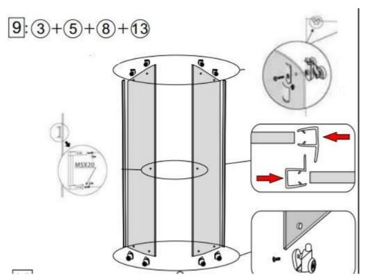
Put wheels on the top and bottom of the curved glass panels. Attach the water seal at the back and the magnetic door strips at the front ends.
